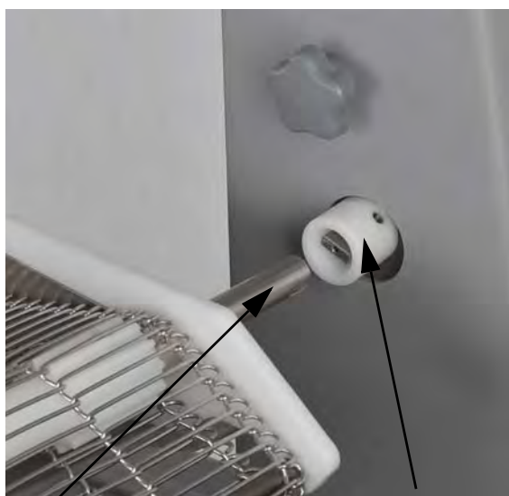
Conveyor Drive Shaft
